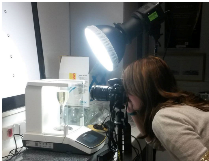
Figure 7. Experimental setup used to monitor simultaneously fluxes of gaseous CO 2 and foaming properties, under standard tasting conditions.
