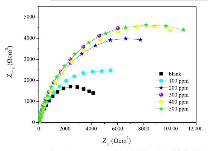
**Figure 6.** Nyquist impedance curves of the Pex 50%–Gx 50% formulation applied to the medium in different concentrations.
