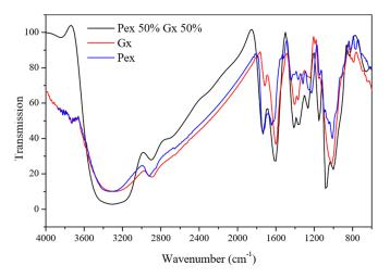
**Figure 4.** Infrared spectra of corrosion inhibitors: extracted pectin (Pex), xanthan gum (Gx), and the Pex 50%–Gx 50% mixture.
