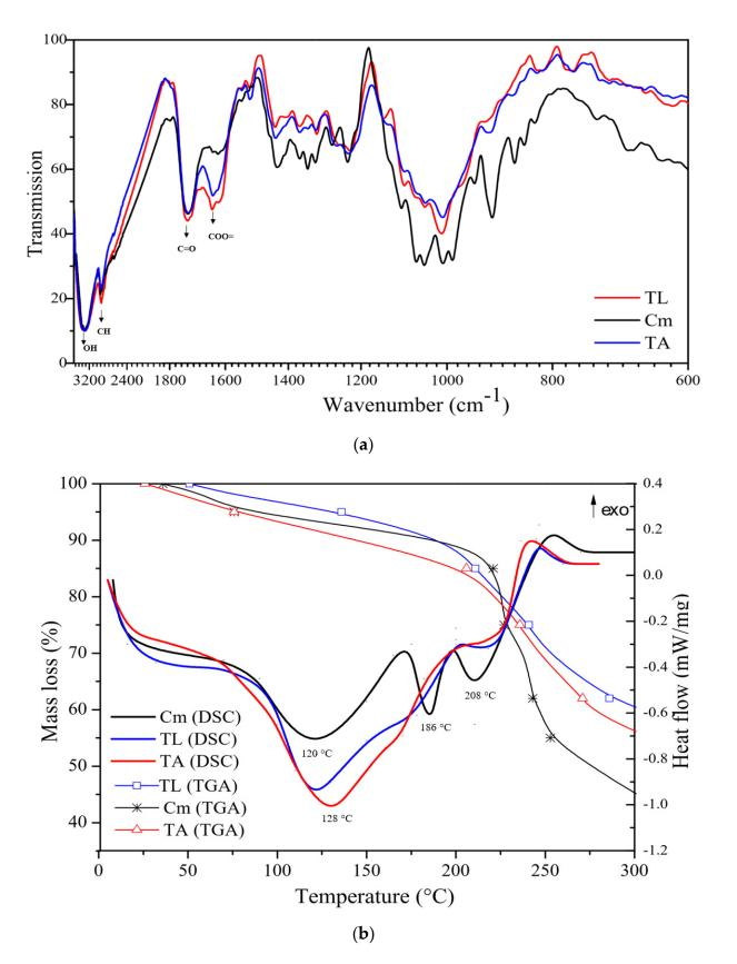
**Figure 2.** Tahiti lime (TL), King mandarin (MK), and commercial pectin (Cm): (**a**) Infrared spectra; (**b**) DSC and TGA thermal analyses.
