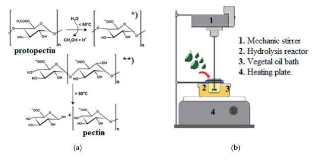
**Figure 7.** (**a**) Pectin hydrolysis mechanism: \* protopectin demethylation, \*\* protopectin hydrolysis (Lim y Cheong 2015, modified by author); (**b**) pectin extraction system.
