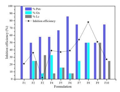
**Figure 3.** Corrosion inhibition efficiency graph for each of the extracted pectin (Pex), xanthan gum (Gx), and lechero plant (Lc) mixture variants in the experimental design.
