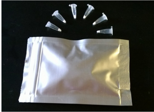
Fig. 1. Lyophilized LAMP reagents for the detection of Coxiella burnetii . The lyophilized reagents were inside a 0.2 ml vial containing Bst DNA polymerase, SYBR green, primers, and dNTPs. Vials were packaged in a zipped aluminum foil bag.
