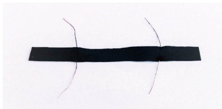
Figure 1. Specimen used for online measurements of electrical conductivity during mechanical deformation.
