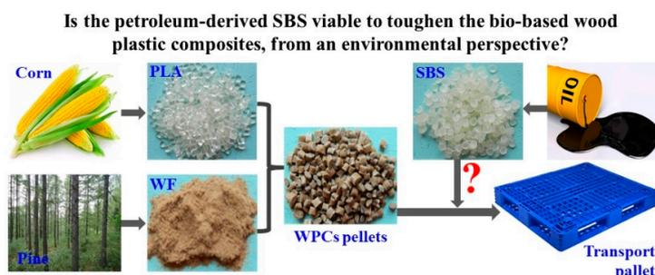
**Figure 1.** Raw materials and manufacture of the polylactide (PLA)-based wood plastic composites (WPCs) toughened with styrene-butadiene-styrene (SBS).
