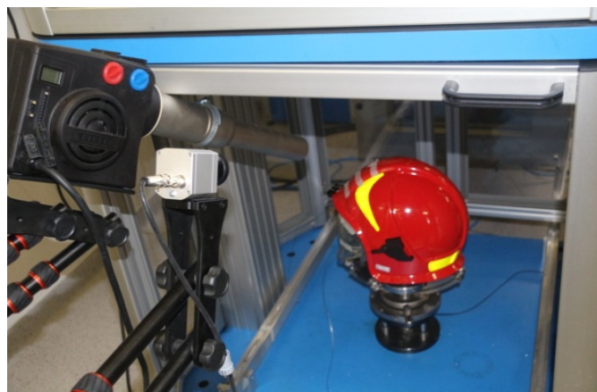
Figure 7. Firefighting helmet CV102 (a helmet shell and some other elements are made of Ultramid PA66-GF25FR) placed on a static head model, located in a measurement track of a drop hammer DFP 1000, which was treated with the hot airflow (air heater HOTWIND SYSTEM).
