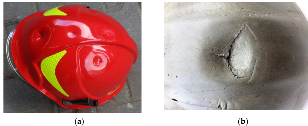
Figure 15. Structural elements of a firefighting helmet after the exposure to the impact loading: (a) a helmet shell after an impact test with the energy of 60 J using an impactor with the diameter of 20 mm at the temperature of 140 °C, (b) an amortizing liner at the impact point in a helmet exposed to the heat load of 140 °C.
