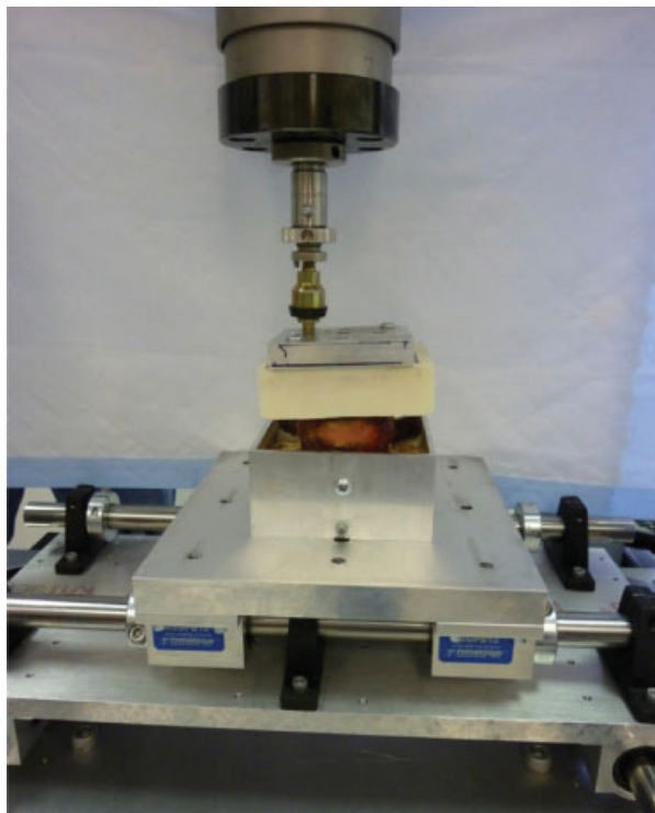
Fig. 2 Experimental setup used for biomechanical evaluation. Specimen is pictured during right lateral bending testing.
