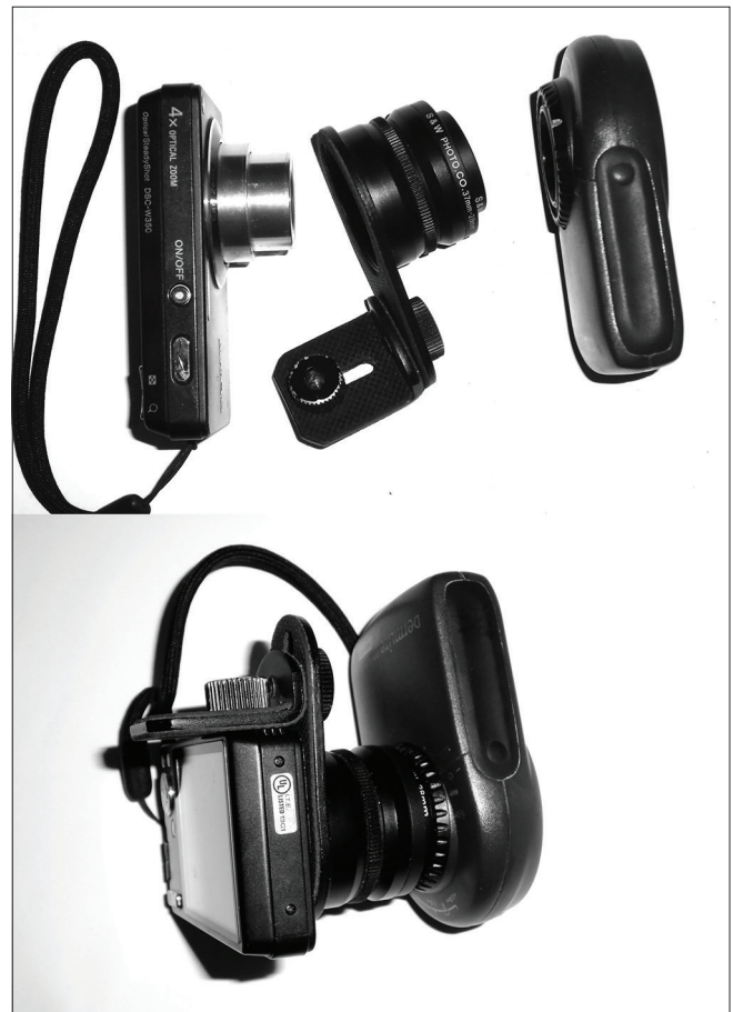
Figure 2: Using screw-on adapters to connect cameras to hand-held units
