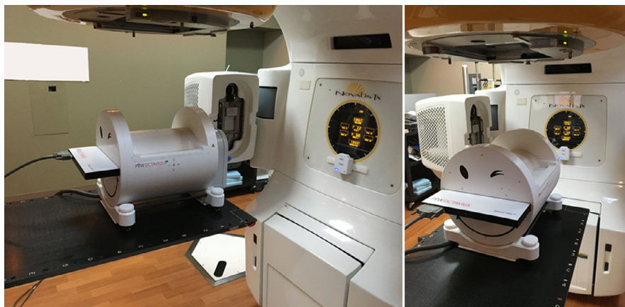
FIG. 1. The Octavius four-dimensional Modular Phantom setup for stereotactic radiosurgery patient-specific quality assurance.
