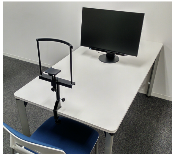
Figure 3. Experimental setup. The participants were sat in front of the display. We explained the experiment and obtained informed consent from each participant. Each participant's chin was placed on the static chin rest. The experiment was conducted after calibrating the eye tracker according to each participant.
