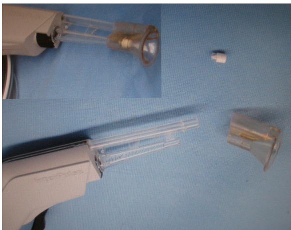
Figure 8 The pulsatile lavage system with disassembled and assembled (inset) components.
