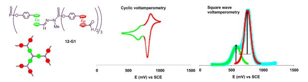
**Figure 12.** Cyclic voltamperometry and square wave voltamperometry of dendrimer **12-G1** in acetone/THF (1:2), versus standard calomel electrode (SCE).
