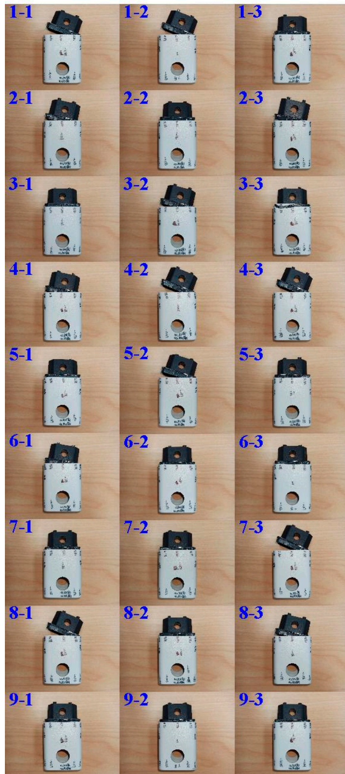
Figure 10. Results of tensile testing for parts fabricated by different process parameters.
