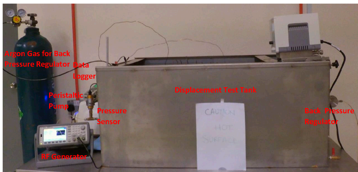
Figure 6. Schematic of experimental setup for nano- \text{Al}_2\text{O}_3 flooding in the presence of EM field, generated by a copper solenoid surrounding the sandpack holder saturated with crude oil.
