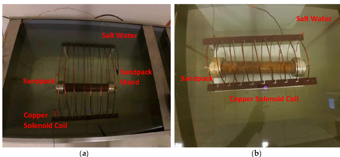
Figure 7. Close-up of test tank comprise of solenoid coil submerged in salt water, while surrounding the sandpack at an experimental frequency of (a) 18.8 MHz and (b) 167 MHz.
