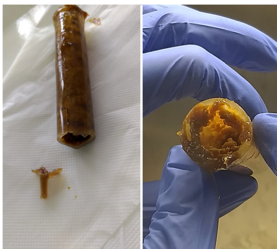
Fig. 4. Left: a syringe filled with grease, broken due to the radiation-induced gas pressure. Right: a section view of the syringe after irradiation. The radiation-induced grease mobility can be observed. The scattering of the grease inside the syringe volume is due to the production of gas bubbles.
