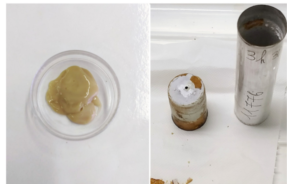
Fig. 10. Left: Krytox 240 AC sample irradiated at 0.97 MGy (3 h and 30 min). Right: the aluminum set-up used for irradiation. The stopper has been corroded by the acid gases evolved.
