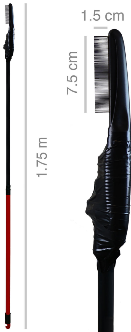
Fig. 1 “Telescopic lice comb apparatus”. Overview and close-up of the metal-toothed lice comb on the head of an aluminum telescopic rod fixed with Tesa® tape
