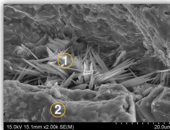
Figure 10. SEM image analysis of cracks in the insulator cement used for 48 years.
