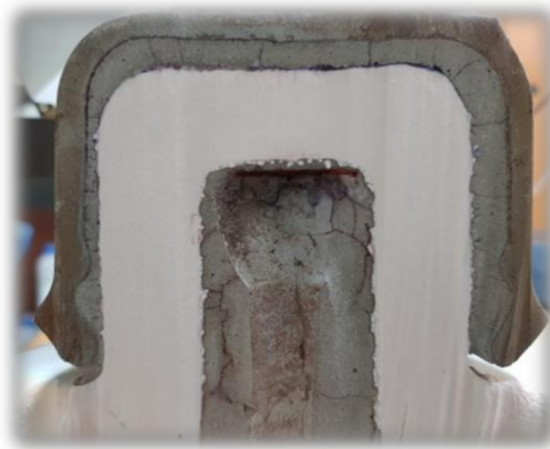
Figure 2. Cement paste surrounding cap of porcelain insulator.
