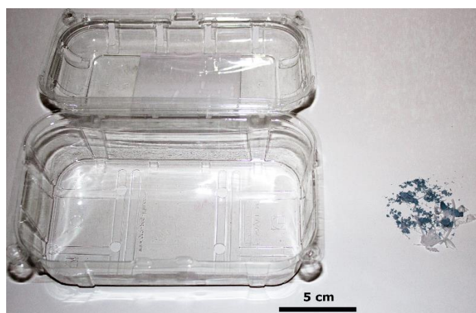
Figure S17: PET clamshell container before and after degradation with PHL7.
