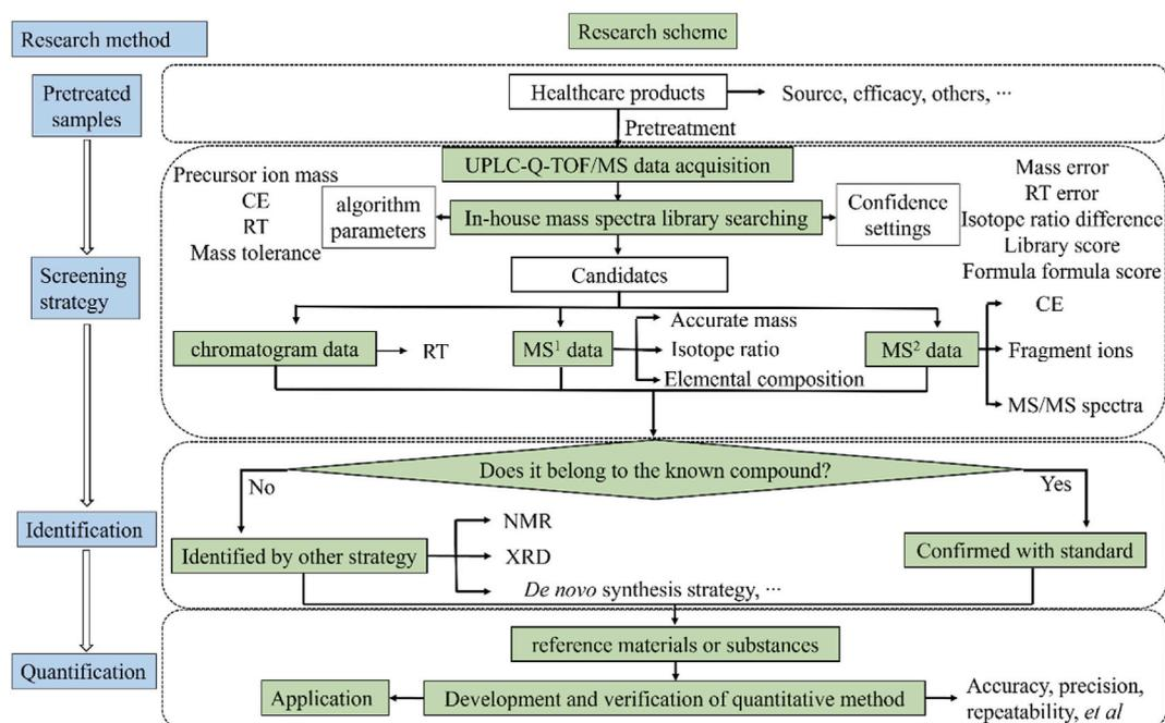
Fig. 2. The systematic technology roadmap for the test of illegally added chemicals in healthcare products.
