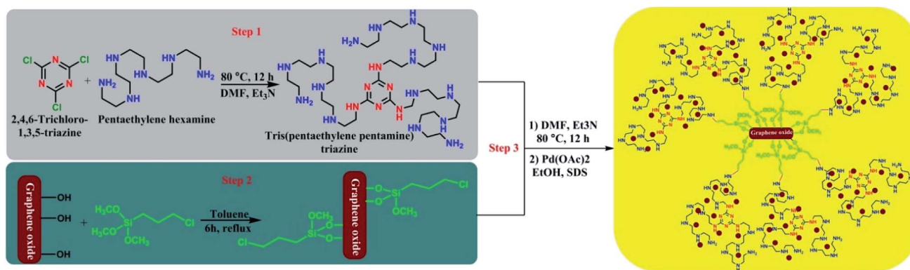
Scheme 2 A synthetic pathway for the synthesis of Pd np -TPEPTA (L) -GO.
