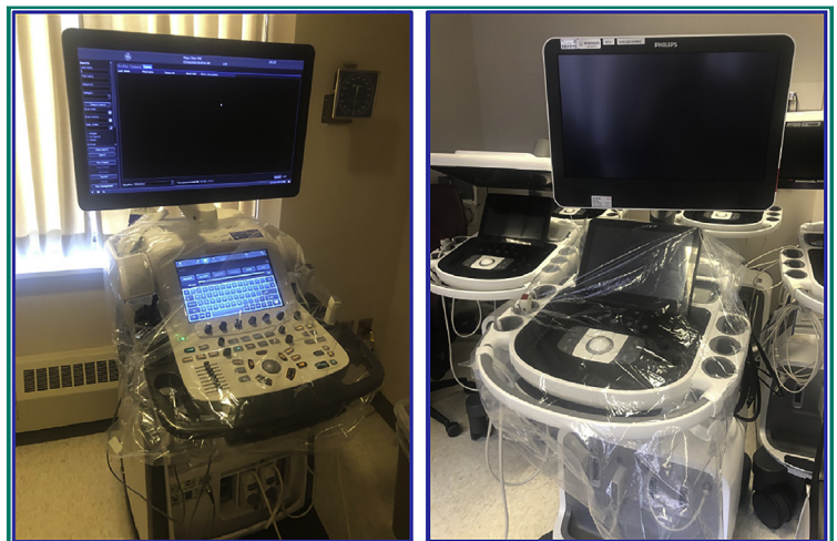
FIGURE 2. Use of an elastic fluoroscopy drape (Genesys, Echolab) placed over the keyboard, controls, and touch panel allows a degree of protection of these critical difficult-to-clean machine elements from contamination. This is recommended for all transesophageal echocardiography and transthoracic echocardiography procedures performed in patients with COVID-19.
