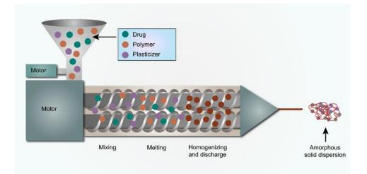
Figure 1. The schematic representation of the HME process.
