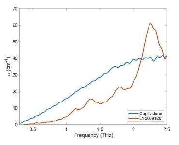
**Figure 6.** The THz absorption coefficient of co-povidone (amorphous) and LY3009120 as measured using THz-TD. Adapted from [159] under Creative Commons Attribution (CC BY) license (https://creativecommons.org/licenses/by/4.0/).
