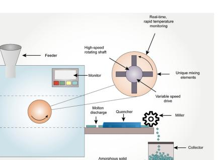
Figure 3. The schematic representation of Kinetisol® process in preparation of amorphous solid dispersions.
