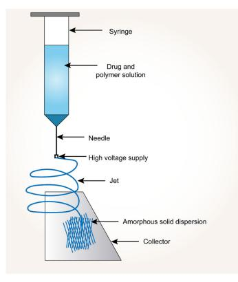
Figure 5. Process of electronanospinning approach.
