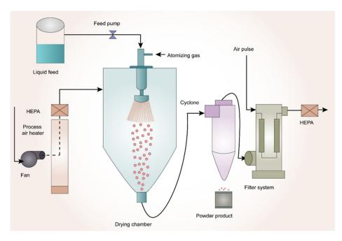
Figure 2. Schematic Representation of Spray-Drying Technology.
