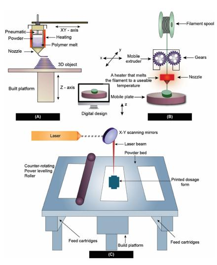
**Figure 4.** 3D-printing techniques used in the preparation of ASD. (**A**) Direct powder extrusion, (**B**) Fused deposition modeling, and (**C**) Selective laser sintering.
