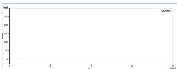
FIGURE 3: Blank chromatogram for specificity by using mobile phase.
