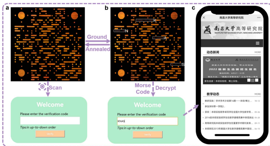
Fig. 5 A complicated QR code. (a) QR code with SQ-OMe and SQ-NMe 2 crystal phases is constructed, and a login window appears when scanning the code with a smartphone. (b) Grinding the QR code leads to the appearance of Morse signals, which are then translated into the letter sequence "KNAS". (c) The input of "KNAS" as the verification code allows access to the target website.
