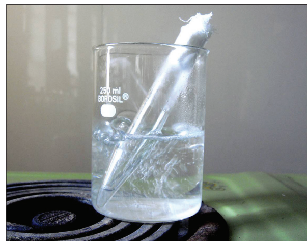
Figure 1: Test tube containing unstimulated saliva sample placed in boiling water bath for approximately 10 min to destroy enzymes
