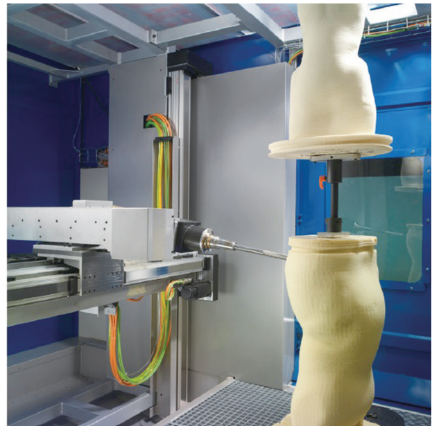
Fig. 2. Carving the mold by using a milling machine [29].
