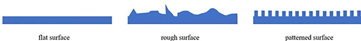
FIG. 5. Comparison between a flat surface, a surface with random roughness, and a surface with specific patterns.
