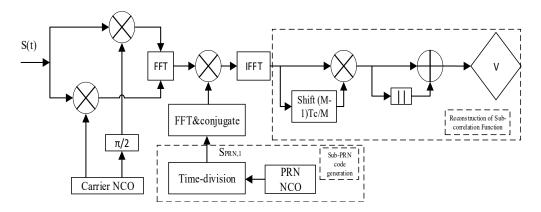
Figure 10. The SRSA acquisition schematic.
