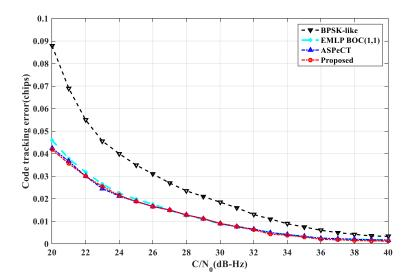
Figure 23. Code tracking error standard deviation of BOC(1,1).
