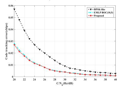
Figure 24. Code tracking error standard deviation of BOC(10, 5).
