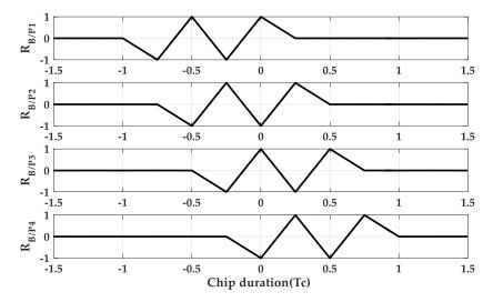
**Figure 8.** The normalized sub cross-correlation functions at M = 4.
