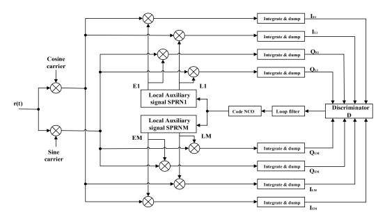
Figure 18. The proposed code tracking loop.
