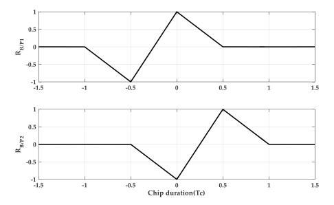
**Figure 7.** The normalized sub cross-correlation functions at M = 2.
