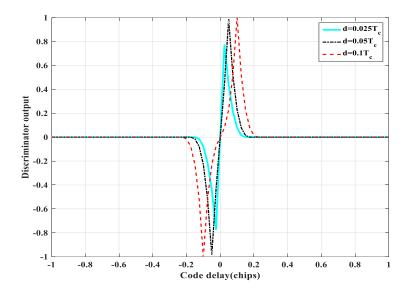
Figure 17. The discriminator curve at different delay spacings of BOC(1, 1).
