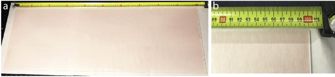
Figure S6. Related to Figure 6. The fabricated large-area QD-based LSCs. (a) The large-area QD-LSC with the dimensions of 100 cm× 30 cm under ambient light. (b) The zoomed view of the scale for better visualization.
