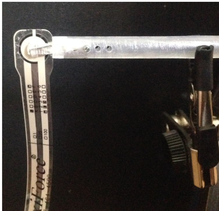
Figure 11 Gripping force measurement experimental setup using Flexiforce.
