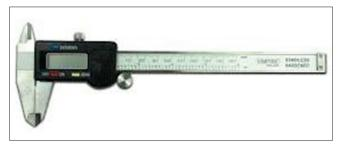
Figure 1: Digital vernier calipers
