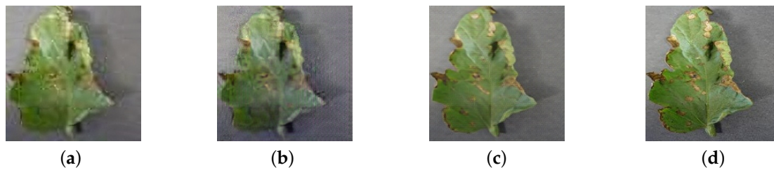
Figure 6. Visual comparison of super-resolution (SR) images generated from three training stages. (a) is from the pre-trained G_{pre} based on ImageNet, (b) is from G_1 after the first fine-tuning and (c) is from G_2 after the second fine-tuning. (d) is the original high-resolution (HR) image.
