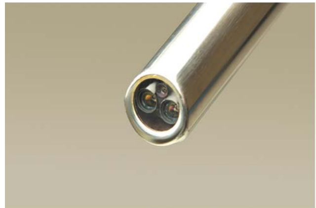
Binocular endoscope compatible with the da Vinci Surgical System.
