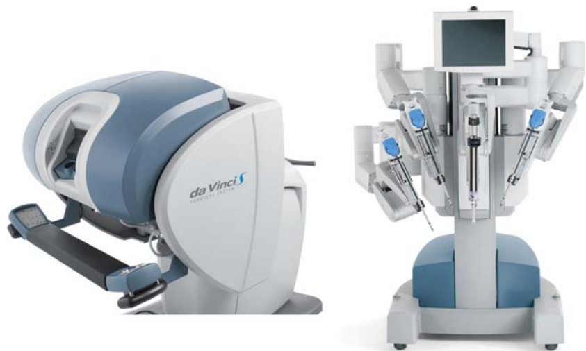
The daVinci Surgical System with the surgeon's console to the left and the robotic arm tower on the right.
