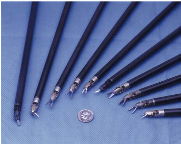
8mm "Endowrist" instruments compatible with the da Vinci Surgical System.
