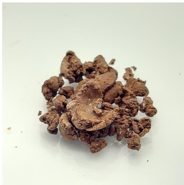
Figure 2. The reaction of sulfur and thraustochytrid oil resulted in thraustochytrid oil polymer exhibiting brown sticky mixture and thickened on cooling.
