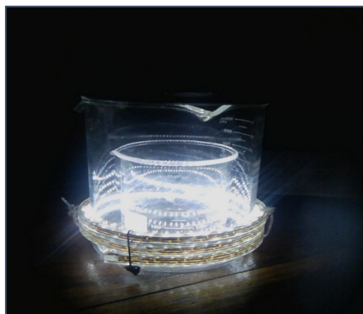
Fig. 1. The LED warm white light coiled around the beaker photoreactor.
