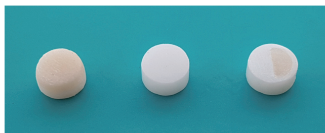
Fig. 1. Tested specimens in the study. Veneering ceramic, zirconia, and 50% zirconia - 50% veneering ceramic.
