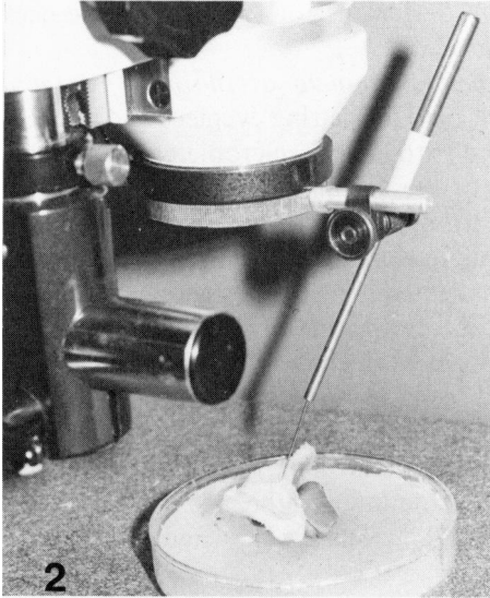
FIG. 2. Acetabular depth measurement. The rim of the acetabulum was levelled by ensuring the pointer made contact on both sides. The adjustable pointer, attached to the microscope head, was contacted first with the rim of the socket ( shown ) then with the lowest level of the acetabular cartilage. Both positions were read off a vernier side scale mounted to the mechanical stage of the microscope. The difference between the rim and the socket floor readings was the depth recorded.
