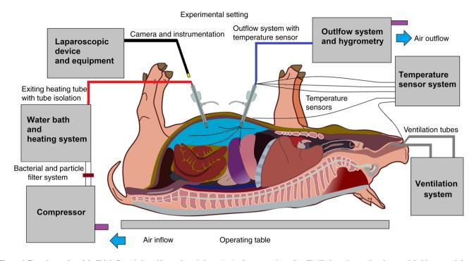
Figure 4. Experimental model of high-flow air-based hyperthermia in an *in vivo* laparoscopic setting. Similarly to the previous box-model, this system is based on a continuous stream of hyperthermic gas with at least two trocars allowing in- and outflow. Furter trocars are inserted to be able to place several temperature sensors at different locations within the abdominal cavity. All sensors and detection systems are monitored throughout the procedure.
