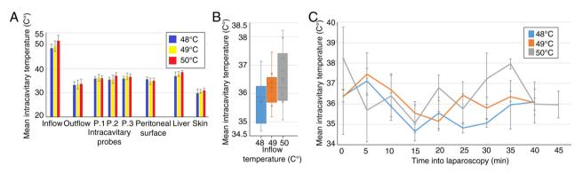
Figure 5. Temperature development during laparoscopy. (A) Mean measured temperatures at various location throughout the 45-min laparoscopy for each swine. (B) Mean intracavitary temperature for each swine throughout the 45 min laparoscopy (Including the locations P1(right upper abdomen), P2 (left upper abdomen) and P3 (lower abdomen). (C) Medium intracavitary temperature development during the 45-min laparoscopy for each swine.
