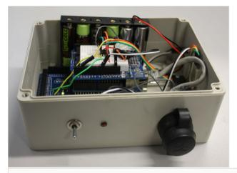
Figure 14. A completed device packaged in a watertight enclosure (with lid removed).
