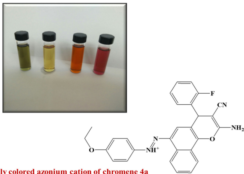
Figure 3. Color change of 4a in the presence of increasing [H^+] in a DMF.
