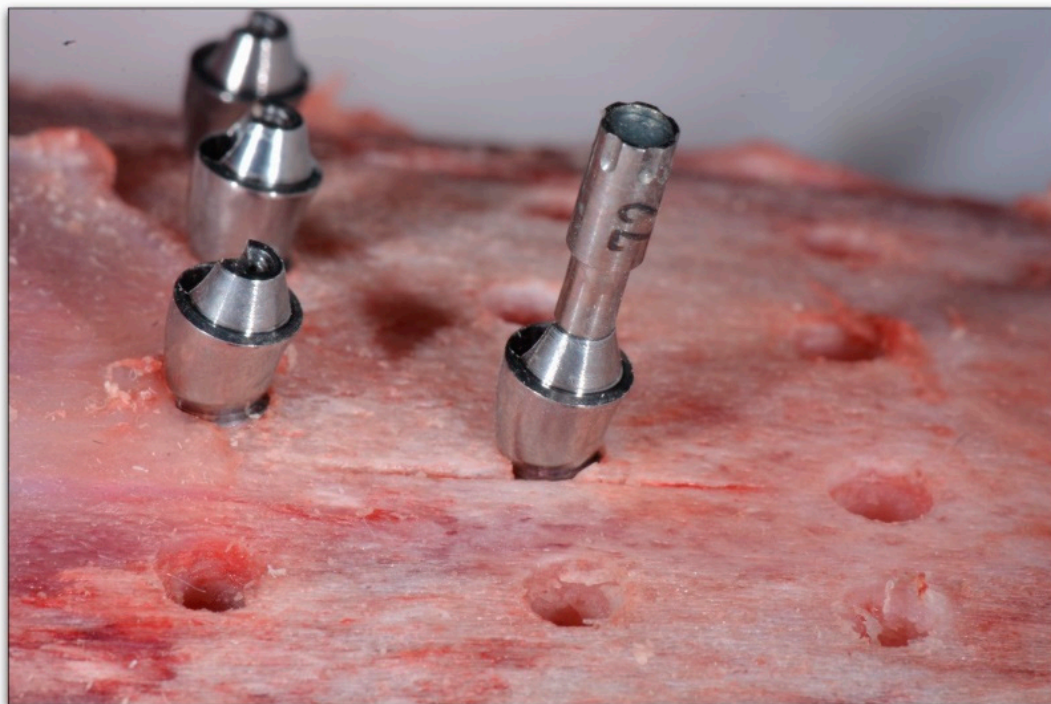
Figure 3. Resonance frequency analysis with Penguin RFA to Multipeg® Reference 72 for the Permanent®, 18° angled abutment with a 2 mm height for Vega® with a 4 mm diameter).
