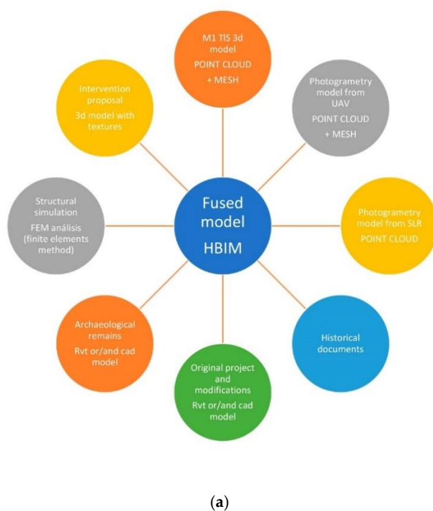
Figure 2. (a) The key to this project is the use of a Historic Building Information Model (HBIM) tool that serves as an articulating element of the different databases obtained, guaranteeing their interoperability with a high level of reliability. (b) Terrestrial laser scanner (TLS) model, processed in Real Work (c) Work in progress of the Structure from Motion (SfM) model in Agisoft Metashape.
