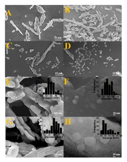
**Figure 4.** (**A**) Micrographs of the pure SBA-15; (**B**–**D**) Images after impregnation on SBA-15 support. (**E**,**F**) Micrographs with the particle size distribution for sample Fe<sub>2</sub>SiO<sub>4</sub>-Co<sub>7</sub>Fe<sub>3</sub>-SBA-15-700-2.0. (**G**,**H**) Image with the particle size distribution for solid Fe<sub>2</sub>SiO<sub>4</sub>-Co<sub>7</sub>Fe<sub>3</sub>-SBA-15-700-0.5.
