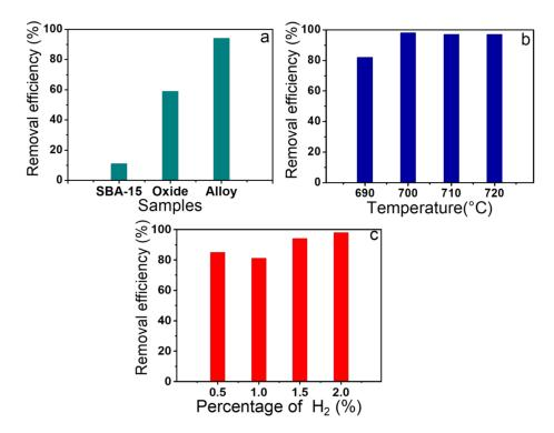
**Figure 6.** (a) Dye removal efficiency for pure SBA-15, oxide, and alloy dispersed on silica matrix; (b) Removal efficiency for the study of the reduction temperature variation; (c) Removal efficiency concerning the study of the effect of H<sub>2</sub> content.
