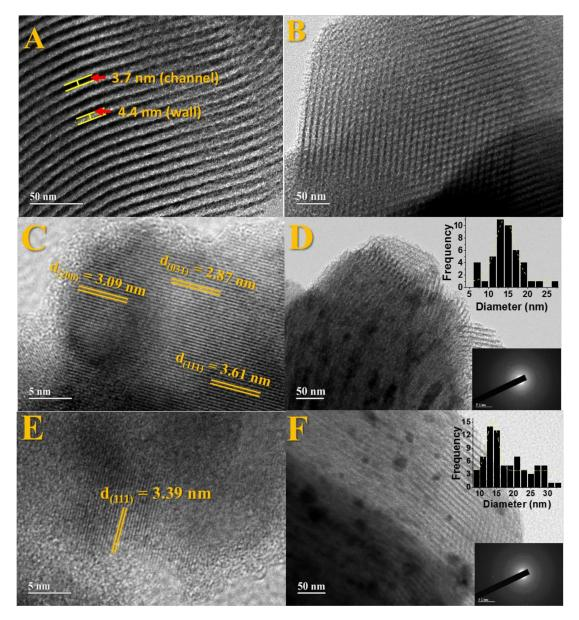
**Figure 5.** TEM images for solids: (**A**,**B**) pure SBA-15, (**C**,**D**) for the solid Fe<sub>2</sub>SiO<sub>4</sub>-Co<sub>7</sub>Fe<sub>3</sub>-SBA-15-700-2.0, and (**E**,**F**) for the sample Fe<sub>2</sub>SiO<sub>4</sub>-Co<sub>7</sub>Fe<sub>3</sub>-SBA-15-700-0.5 using different approximations. The figures inserted above are related to particle size distribution and below concerning the selected area electron diffraction (SAED).
