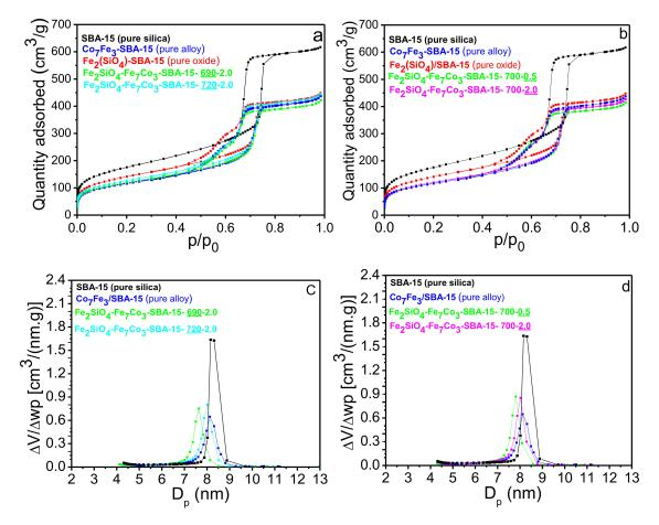
**Figure 3.** (a)  $N_2$  isotherms for pure SBA-15,  $Fe_2SiO_4$ -SBA-15,  $Co_7Fe_3$ -SBA-15, and the two extremes of reduction temperature studied; (b)  $N_2$  isotherms for the pure SBA-15,  $Fe_2SiO_4$ -SBA-15,  $Co_7Fe_3$ -SBA-15, and the two extremes of hydrogen quantity studied; (c) and (d) Pore diameter distribution for the different materials described in Figure 3a,b.
