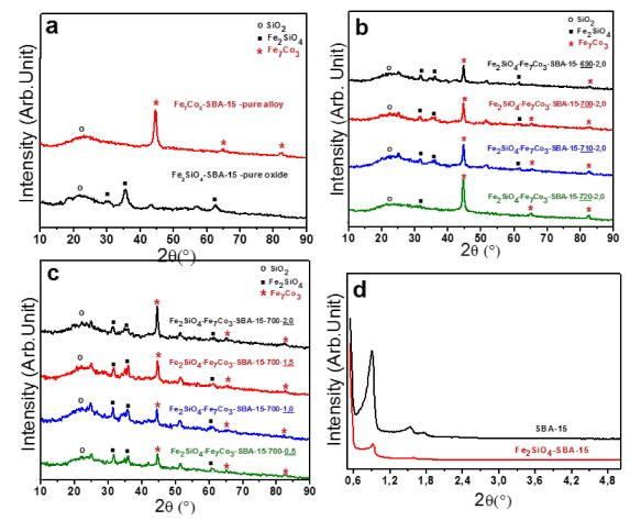
**Figure 1.** (a) Diffractograms of pure oxide ( $Fe_2SiO_4$ -Santa Barbara Amorphous (SBA)-15) and pure alloy ( $Co_7Fe_3$ -SBA-15); (b) Diffractograms concerning the influence of reduction temperature; (c) Diffractograms referring to the influence of H<sub>2</sub> content; (d) Low-angle diffractograms for the support (SBA-15) before and after impregnation.
