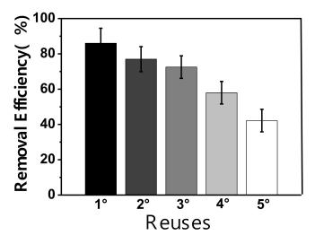
Figure 7. Reuse tests for methylene blue dye removal using the sample Fe<sub>2</sub>SiO<sub>4</sub>-Co<sub>7</sub>Fe<sub>3</sub>-SBA-15-700-2.0.
