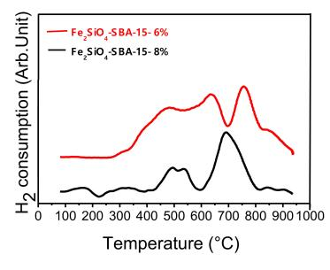
Figure 2. Temperature-programmed reduction (TPR) curves for the pure oxide dispersed on the SBA-15.
