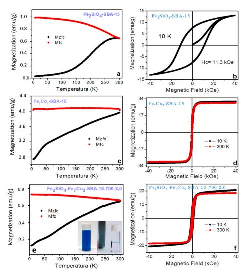
**Figure 8.** Magnetic properties for different samples. (**a**,**c**,**e**) magnetization zero field cooling (Mzfc) and magnetization field cooling (Mfc) magnetization curves; (**b**,**d**,**f**) Hysteresis cycles from vibrating sample magnetometer (VSM) analysis. The photo inserted in Figure 8f represents the nanocomposite separation by the application of a magnetic field after adsorption.
