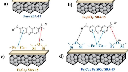
**Scheme 1.** Mechanistic proposal for the methylene blue adsorption on the surface of different composites indicating the different types of interaction. (a) pure silica matrix; (b) oxide dispersed in SBA-15; (c) alloy supported in SBA-15; (d) oxide and alloy mixture dispersed in SBA-15.
