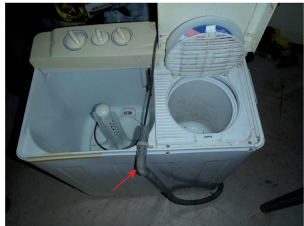
Fig. 2. “Danby” clothes washing machine. The compartment on the left is used to agitate and clean clothes in water and detergent. The compartment on the right is a “spinner” that uses centripetal forces to remove water from clothes. You can see in this image that the water drainage tube (identified by red arrow) is re-feeding into the agitation compartment to “recycle” water for multiple loads of laundry.
