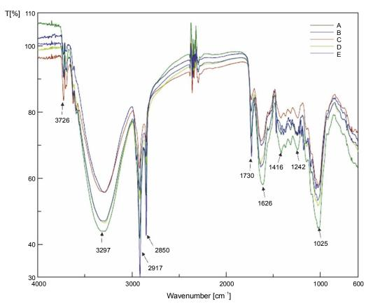
Fig. 2. FTIR spectrum of powdered samples of *Centella asiatica* obtained by different drying techniques: A) freeze drying, B) microwave drying, C) oven drying, D) shade drying, and E) solar drying
