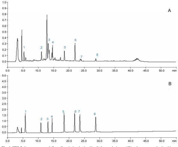
Fig. 1. HPLC chromatogram of *Centella asiatica* obtained by A) freeze drying and B) reference standards; chlorogenic acid (1), rutin (2), madecassoside (3), asiaticoside (4), quercetin (5), kaempferol (6), madecassic acid (7), and asiatic acid (8)
