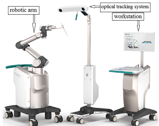
Fig. 1 TiRobot, mainly composed of a workstation, an optical tracking system, and a robotic arm (Photo provided by Beijing Tianzhixing Medical Technology).
