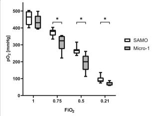
**Fig. 2** Oxygen partial pressure. ECMO began with FiO $_2$  at 1.0, and the pO $_2$  was measured after 15 min – the FiO $_2$  was adjusted to 0.75, 0.5 and 0.21 respectively. Values are expressed as medians with Min/ Max values, \* indicates that values are statistically significant different ( $\rho$  < 0.05), tested by using the Wilcoxon–Mann–Whitney test
