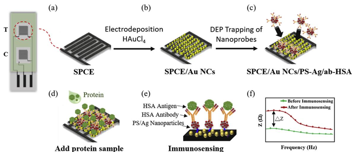
Fig. 4. Schematic illustration of systematic protocol for immunosensor fabrication and operation. (Reprinted with permission from Ref. [18] Copyright 2019: Elsevier.).
