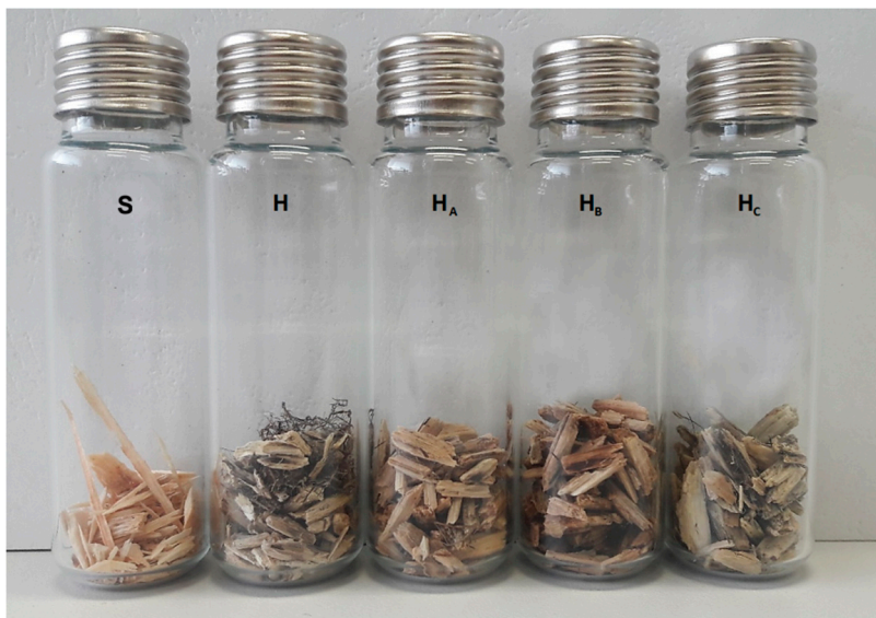
Figure 1. The samples closed in vials ready for GC-MS analysis—visual color change: (S—spruce strands, H—untreated hemp shive, H A —hemp shive after tartaric acid treatment, H B —hemp shive after citric acid treatment, H C —hemp shive after sodium bicarbonate treatment).
