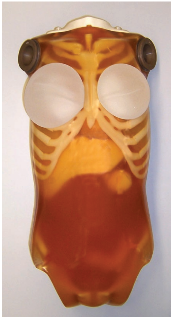
FIGURE 1. Image of the phantom with 340 ml implant size on the right and 500 ml implant size on the left.
